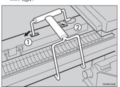
There is the green lever (1) on the left side of the fusing unit. While pressing the green lever to the left, slide the fusing unit out slowly using the removal tool.
