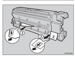
Align the new development unit to the rail of the printer. Slide the development unit into the printer until it makes a click as it locks into place.
