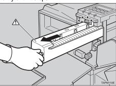
Take the removal tool from the Type 4500B box, and attach the tool to the fusing unit.
