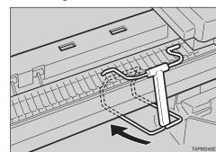
② Insert the removal tool into the top hole on your side (1), and then into the hole on the printer side (2).
