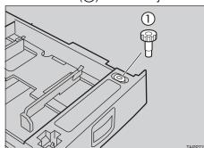
Remove the screw inside of the front cover (1) by turning it counterclockwise to release the fusing unit
