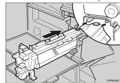
At the right side of the printer, remove the tape on the left and right sides of the black sheet, and then pull out the sheet using both hands.
