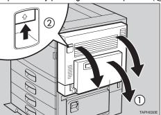
Open the right cover by pushing the catch upwards.
