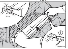
While pressing down on the corner of the transfer unit indicated by the arrow(1), return the green lever (2) to its original position to lock the transfer unit in place.
